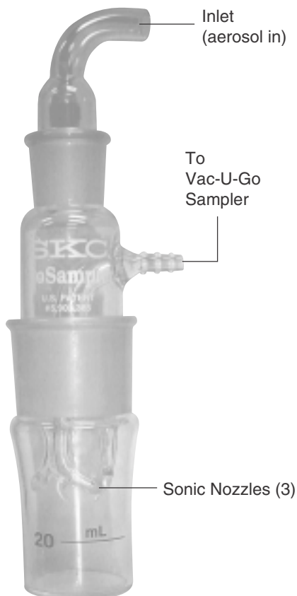
Figure 1. BioSampler with 20 ml vessel (5 ml vessel available)
